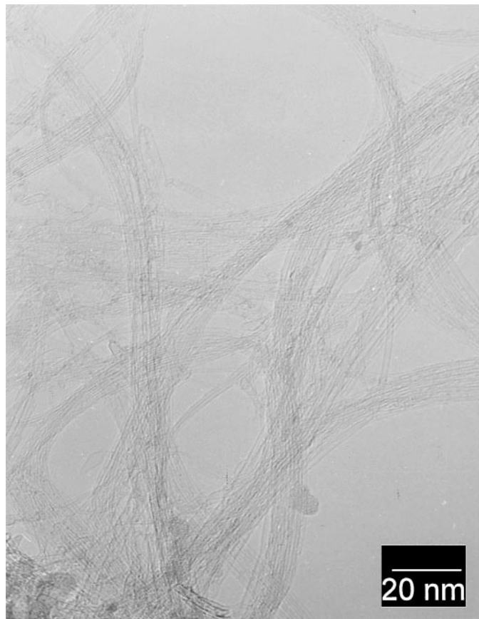
FIG. 17. TEM images showing SWNT produced by CO disproportionation on a Co:Mo (1:3)/SiO 2 catalyst.
